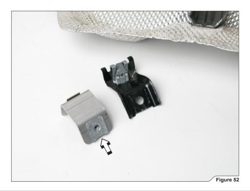
6. Tighten the Akrapovič brackets onto the muffler heatshield, using stock bolts. Slide the Akrapovič M6 press on nuts on the other side of the brackets (Figure 53).
