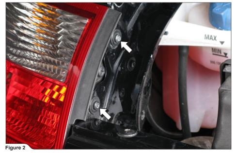
3. For Slip-On, Sports Cup, Evolution, Evolution-Race and SlipOn-Race: undo the lights connectors and remove the tail lights (Figure 3).
