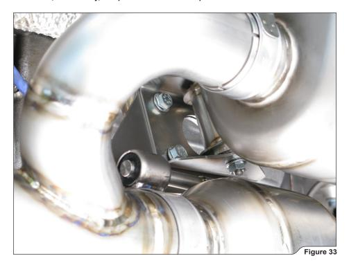
16. For Slip-On, Sports Cup, Evolution, Evolution-Race and SlipOn-Race: hang, center and align (see the reference measurement in figure) the muffler (Figure 34). Tighten the muffler clamps to a specified torque.
