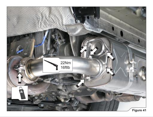
23. **For Evolution-Race:** align the link pipes and tighten all M8 nuts on Akrapovič muffler flanges and bolts on metal clamps to a specified torque **(Figure 42)**.
