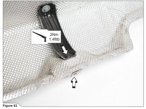
7. After installation of the muffler heatshield and rear bumper onto the vehicle, tighten the bumper onto brackets, using Akrapovič M6x16 bolts and washers. Bend the edge of the heatshield so, that the clearance between heatshield and muffler is at least 10mm (Figure 54).
