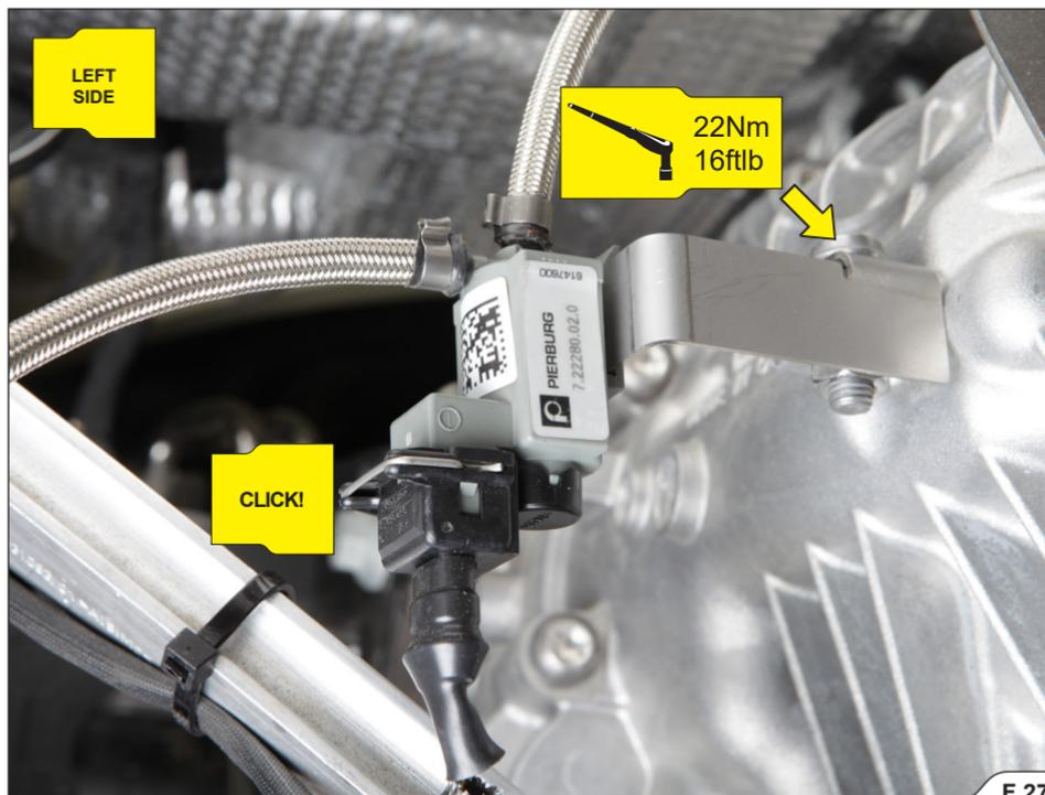
11. Unscrew the marked nut and attach the right electromagnetic valve onto the sub frame, using marked stock nut and connect the right connector (F 28).
