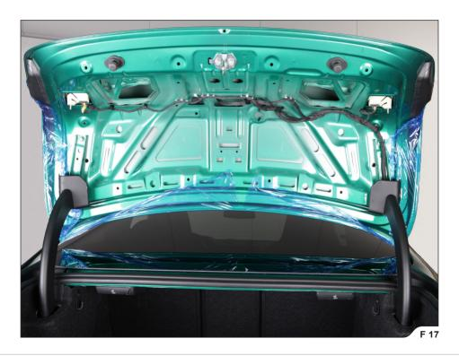
6. Protect the complete rear end of the car (rear windscreen, rear wheel arch panels, rear bumper and boot opening) in such a way, the boot lid can be opened and closed, using protective cloth or equivalent (F 18, 19).
