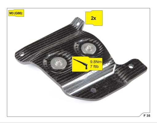
15. Install and carefully align reinforcement plates against the boot lid, adjust the bushings in such a way, they touch the outer shell of the lid and make sure they are secured in the centers of the holes (M4: F 36, 38; M3: F 37, 38).
