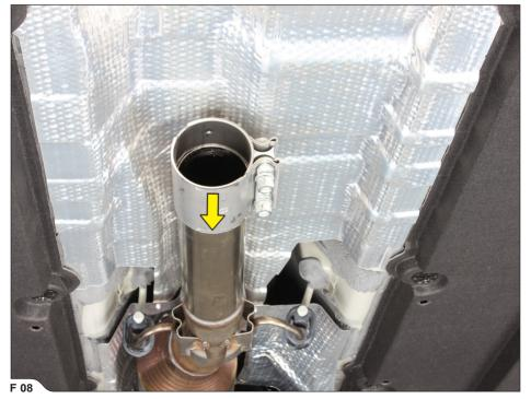
Carefully install the Akrapovič system onto the vehicle; attach all rubber brackets onto the chassis, align the muffler in respect to the chassis, align and center the double clamp in the middle of the pipe joint and tighten the clamp to the specified torque (F 09, 10, 11, 12, 13).
