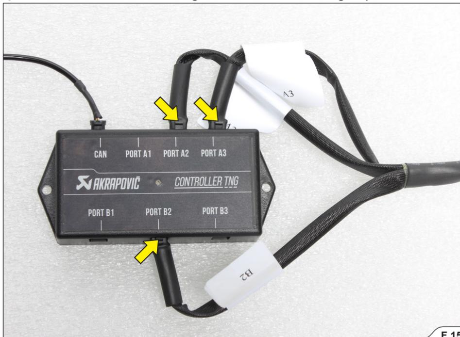
**!** IMPORTANT: make sure to secure the harness in such a way, that it won't touch any hot or moving parts of the vehicle!
