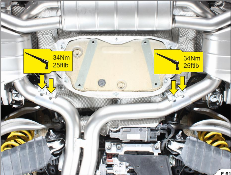
13. Connect the Akrapovič Control Kit connectors to the both exhaust valves (F 62).
