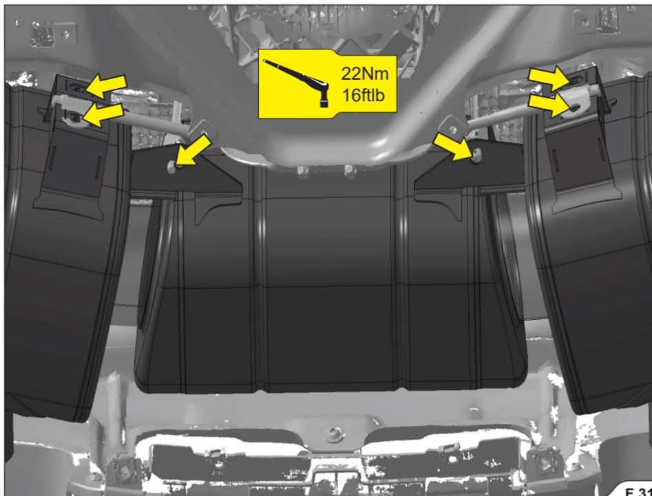
10. Reinstall the middle part of the diffuser; check vehicle manufacturer manual for correct procedure and tightening torques (F 32).
