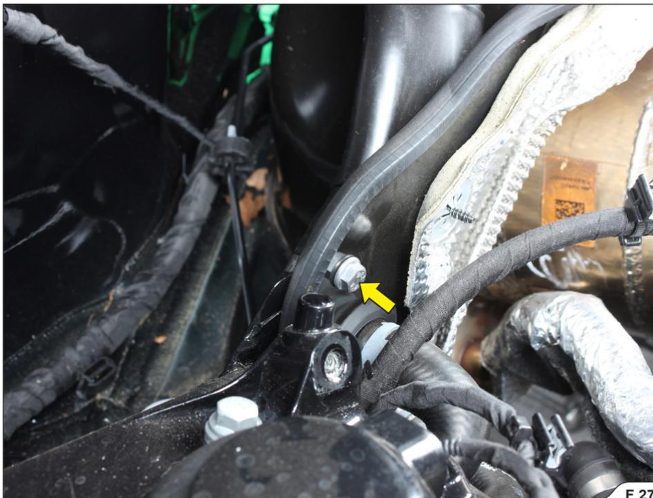
9. **For vehicles with OPF/GPF only:** undo the market clamps, remove the tubes off the sensor, disconnect the sensors' electrical connectors, unscrew the marked bolts and remove sensors, on both sides of the engine compartment (F 28).
