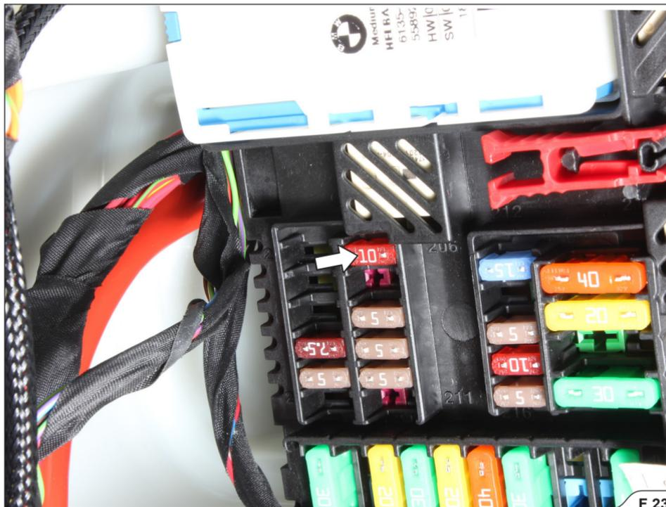
4. Install the original 10A fuse into the Sound Kit's power supply connector and plug the connector into the F206 fuse spot in the fuse box (F 24, 25).
