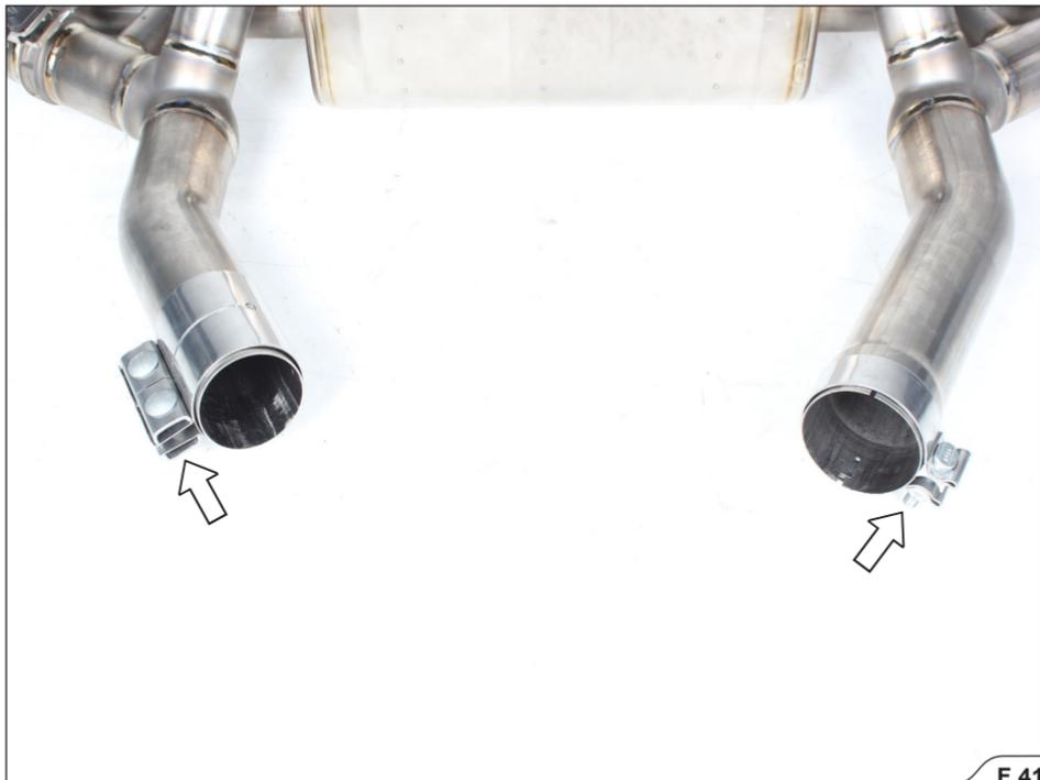
**!** IMPORTANT: unscrew the double clamp's nuts enough, to be able to slide the clamp completely onto the pipe (F 42)
