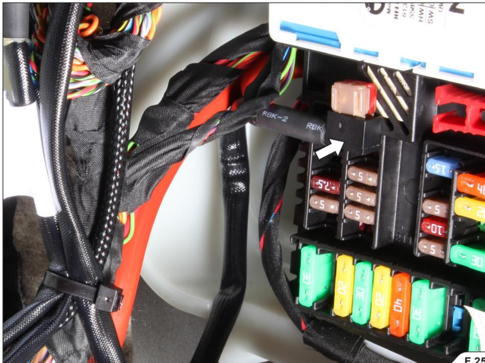
5. Lead the exhaust valves' wiring harnesses, as shown, through the chassis opening, to the left and right exhaust valves' actuators and secure the wiring in place, using tie wraps from Akrapovič installation kit; correctly attach the harness's rubber grommet into the chassis opening (F 26, 27, 28, 29, 30).
