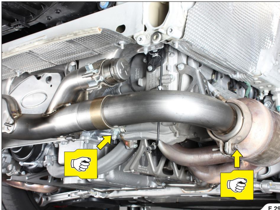
9. **For Slip-On Race only:** align the Slip-On Race system in respect to the chassis and tighten it to the muffler brackets, using brackets and bolts from Akrapovič installation kit (**F 30, 31**).
