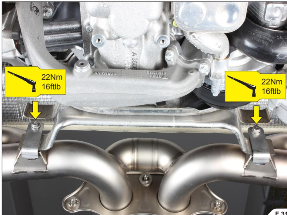
10. **For Slip-On Race only:** align all the clamps as shown and tighten them to the specified torques (F 32).
