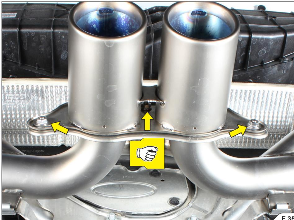
12. **For Slip-On Race only:** reinstall all dismantled stock parts; check vehicle manufacturer manual for correct procedures and tightening torques.
