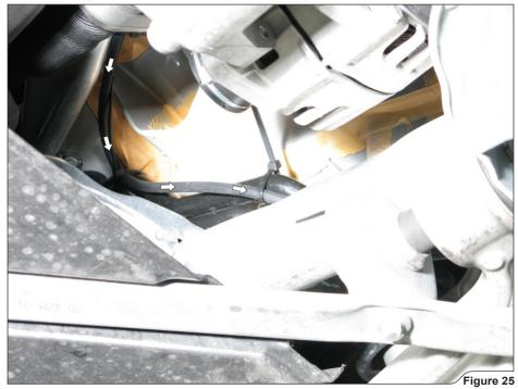
WARNING: direct and secure (use additional plastic tie wraps) the rubber vacuum hose in such a way, that it doesn't touch any hot or moving parts of the vehicle!
