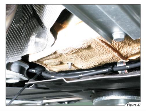
WARNING: direct and secure (use additional plastic tie wraps) the rubber vacuum hose in such a way, that it doesn't touch any hot or moving parts of the vehicle!
