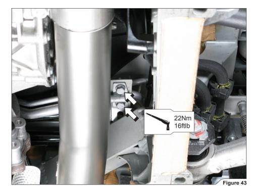
Slide the Akrapovič Muffler onto the Akrapovič Middle Pipes, position the muffler correctly in respect to the vehicle and tighten stock brackets' bolts and Akrapovič connection clamps to a specified torque (Figure 44, 45, 46).
