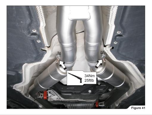
20. Push the collector and muffler pipes together, adjust the clamps and tighten them to a specified torque (Figure 42).
